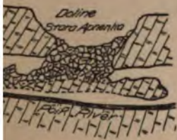
— Cross section of the doline formed by inbreak of a cavern. The Stara Apnenka doline, Carniola (after Martel).
